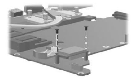
Where used: 2 screws that secure the Bluetooth module to the system board
